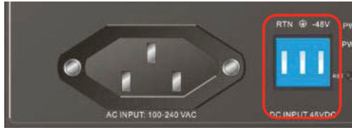
Figure 4-6. Inserting the DC power cable into the DC terminal block to power on this switch.
